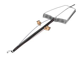
**9.** S-fold the left side of the canopy under the centre of the parachute, then S-fold the right side of the canopy onto the centre of the chute. Keep the canopy neatly folded in place using sandbags or books.
