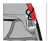
7. Tuck away the risers excess ( without making knots ) under one single flap :
