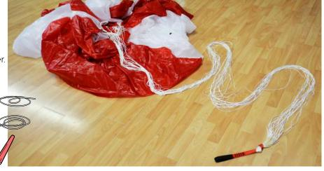
b. Attach the parachute on a fixed point to keep it stretched and under tention.
