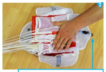
Position the POD's elastic loop opposed to the suspension lines.
