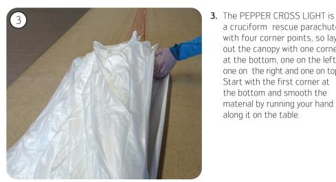
a cruciform rescue parachute with four corner points, so lay out the canopy with one corner at the bottom, one on the left, one on the right and one on top. Start with the first corner at the bottom and smooth the material by running your hand along it on the table.
