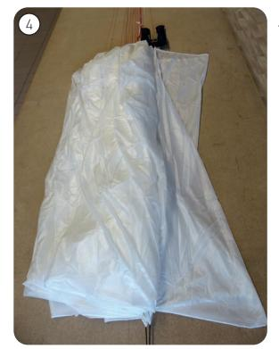
4. Pull the base from one line attachment point to the next along the seam to the side you are sorting and smooth the crossed panel. A line separator and a weight will help to secure the already sorted lines.
