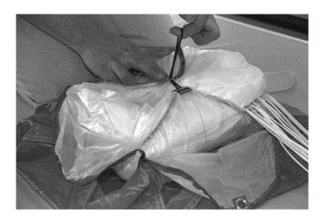
**16.** Pull the elastic band through the eyelet of flap no.3 and no.4.
