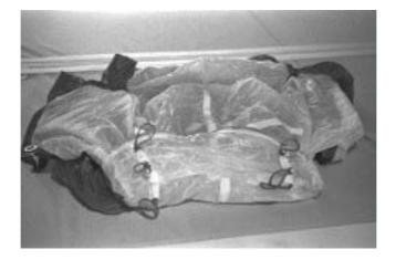
**11.** Now fold the dome with a first S-fold from the base edge (note the container size).
