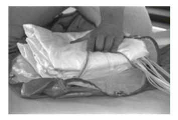
15th First pull the elastic band through the eyelet on flap # 1, then through the eyelet on flap # 2.
