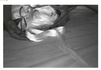
19th The last meter of line is laid in eight loops and fixed with the last two elastics.
