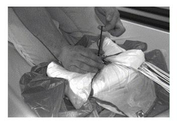
**17th** Pull a line loop (approx. 3 fingers wide) through the elastic loop and "close" the inner container.
