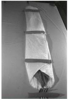
**9.** Pull the packing cord (folding aid) out of the packing loops!
