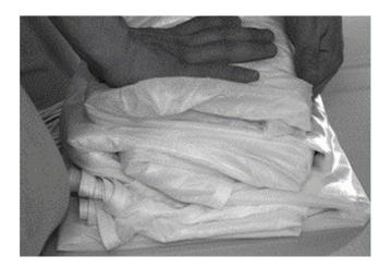
**13.** Place the throwing container on the fabric package so that the top end of the cap (with the packing loops) comes to rest on the container bottom. The container flap number 1 with the elastic band points in the direction of the lines.
