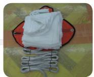
Before closing the pod, we recommend to turn the parachute over so that the skirt is uppermost and closest to the clover leaves. Close the deployment bag around the parachute, neaten the edges to ensure that the parachute is contained completely within. Use the remaining free line to secure the main loop of the deployment bag.
