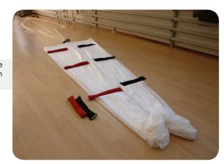
8 Completely fold the gores of one side over to the other so that all of the gores are on top of each other.
