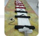
Now arrange the lines keeping them neat and under tension. Use figure of 8 folds and elastic bands around the loops to arrange the lines neatly. The figure of 8s should be made to the same width as the deployment bag. Leave approximately 0.5m of line free at the end before the bridle.
