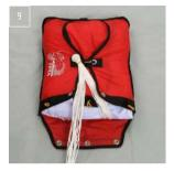
Secure the suspension line using the middle elastic band.
