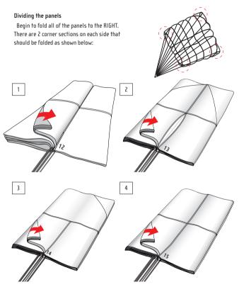
IMPORTANT: The 2 corner sections on each side should be folded as shown.
