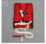
There should be around 40cm of suspension line remaining to connect with the harness.
