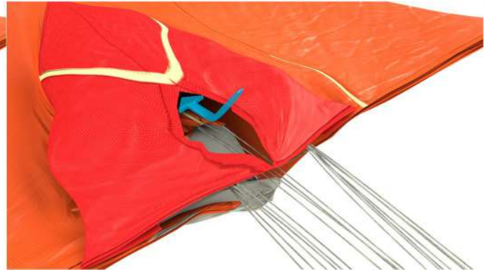
Picture Remedied apex and centring the centre lines
