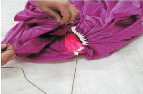
5.3. Insert any spare rope into 18 loops in the middle of the seams connecting the gores. Attach this rope to any fixed point. Attach the main bridle to another fixed point, tensioning the rigging lines until they are straight with a force of approximately 5 kg.
