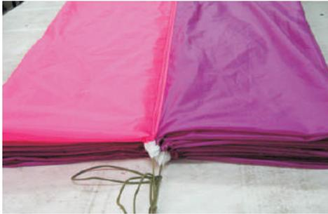
5.6. Make sure that each gore is folded properly and the seams of each bore are parallel, being straight and slightly tensioned. To achieve the desired effect you may use little sand bags.
