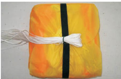
5.14. On one of the big flaps there is a rubber loop, attached to it. Close this flap first. Then close flaps starting from the opposite to the flap with rubber loop by pulling the rubber loop through the grommets of flaps, from below. Pull the rigging lines through this rubber loop, leaving a loop of lines about 3-5 cm.
