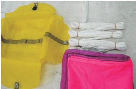
5.10. Group the rigging lines in an S-form along the canopy base. Fix the lines with six rubber bands.
