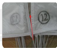
9 Now fold the right hand side underneath using 'S' folds to the width of the deployment bag.
