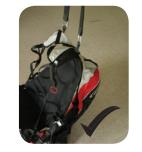
Maillons must be closed tightly - finger tight then 1/2 a turn with pliers is sufficient. Do not overtighten.
