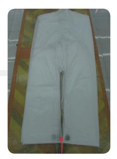
8 The parachute should look as shown with the corner vent of panel 12\* in the middle and on top. The corner vent of panel 1 should be in the middle underneath.
