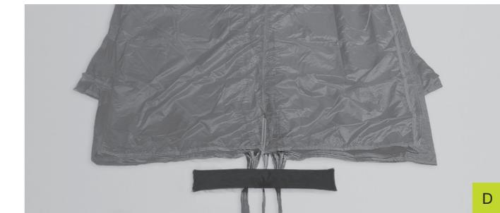
Follow the outer suspension lines to find the centre panels and begin the folding process. ([Image E](#))
