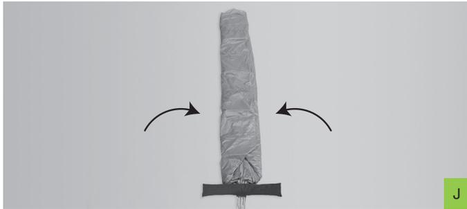
Fold the canopy in an accordion or “Z” shaped folds, so that it fits into the inner deployment bag. If possible, adjust the folds so that those at skirt level are slightly shorter and those at the top of the canopy are slightly longer. The OCTAGON 2 rescue fits well if there are 4 folds. (Image K and L)
