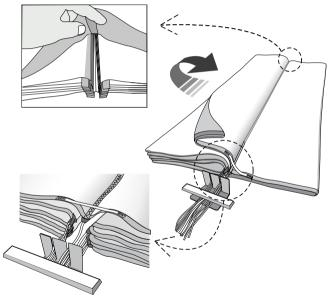
After folding all the panels, check again that the centre seams and the inside of the panels are even and lie in the same direction.
