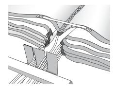
And follow the outer suspension line to find the centre panels to start folding with.
