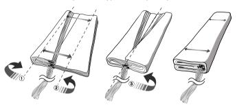
Fold the canopy in an accordion or "5" shaped fold, so that it fits into the inner deployment bag. If possible, adjust the folds so that those at the skirt are slightly shorter and those at the top of the canopy are slightly longer.
