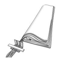
By folding each panel to the left side of the suspension lines again one by one, check carefully that each panel is laid evenly and without creases. Check the centre seams and inside the panels, too.
