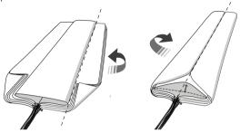
Fold the canopy in half along the central axis and open the skirt of the wind channel to make a mouth.
