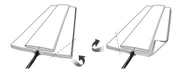
Fold the outside edges onto the wind channel as shown below, but don't overlap them.
