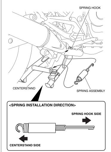
• If the spring assembly is too hard to install, remove the centerstand shaft. First hook the spring assembly, then install the centerstand shaft.
